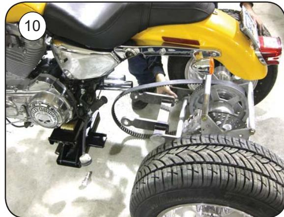
11. Install swing arm pivot shaft and allen bolt, use blue loctite.
