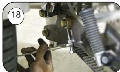
19. Tighten jam nut on adjuster bolts.
