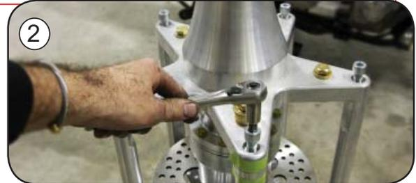
3. If you have a 1999 and earlier Softail with a pulley or sprocket that has a center hole with a diameter of approximately 1.980" (50.292mm) then your pulley or sprocket will need to be machined. Install tool as shown using supplied bolts. Place back side of tool onto lathe chuck. Use boring tool to expand the diameter of the center hole. Measure frequently while boring until the diameter of the center hole is 2.212" (56.185mm). If your Softail is 2000 and later go to next step.
