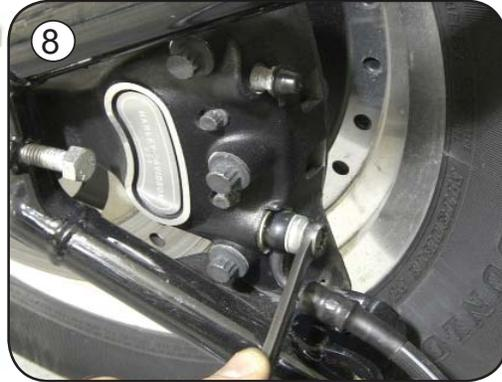
**TIP** Once the brake line is unhooked from caliper, make sure to hang line upright so no fluid leaks out and no air gets trapped in the brake line.
