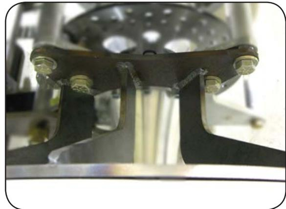
★ *Note: side with more space from bolt holes to edge of fender goes toward the front.*
