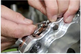
3. Remove brake pad retainer bolt (brakes should fall out)
